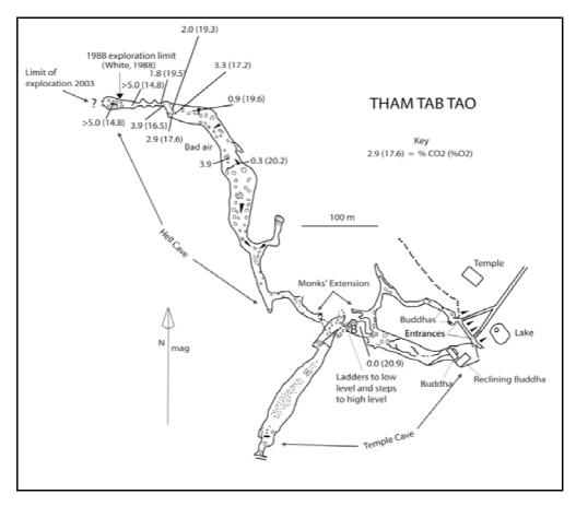
**Figure 2.** Survey of Tham Tab Tao Survey drawn using hand compass and estimating distances. Dual numbers represent carbon dioxide and oxygen concentrations (%) measured in situ. Bad air (high CO<sub>2</sub>; low O<sub>2</sub>) is present in the NW 'Hell Cave' section of Tham Tab Tao. Adapted from White, 1988, courtesy of BCRA.
