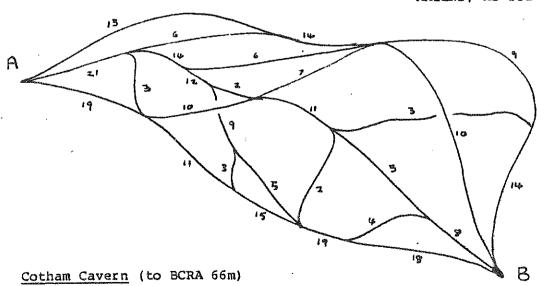
The plan shows a cave system with water entering at sink A and leaving at rising B. The figures by the passages show the maximum possible flow of water (in volumes per unit time) through those passages. (Assume an even down-gradient from the sink to the rising.)
