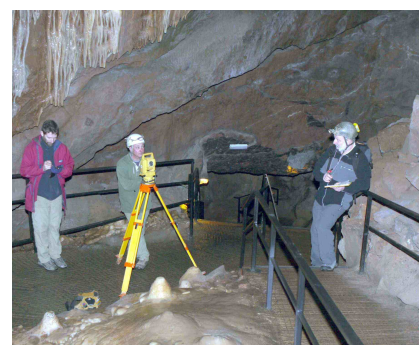
Using the Leica Total Station in King Solomon's Temple
