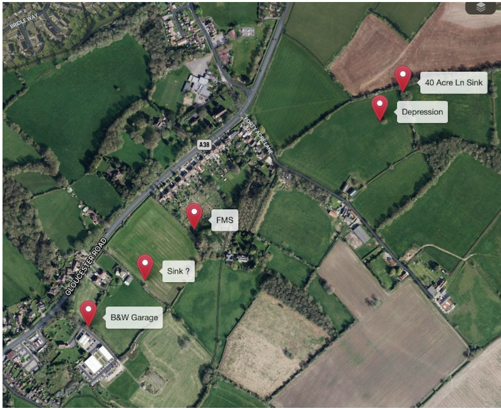
Figure 3. Diagram showing location of stream sinks in Alveston - Note the linear orientation along the boundary of the carboniferous limestone.
